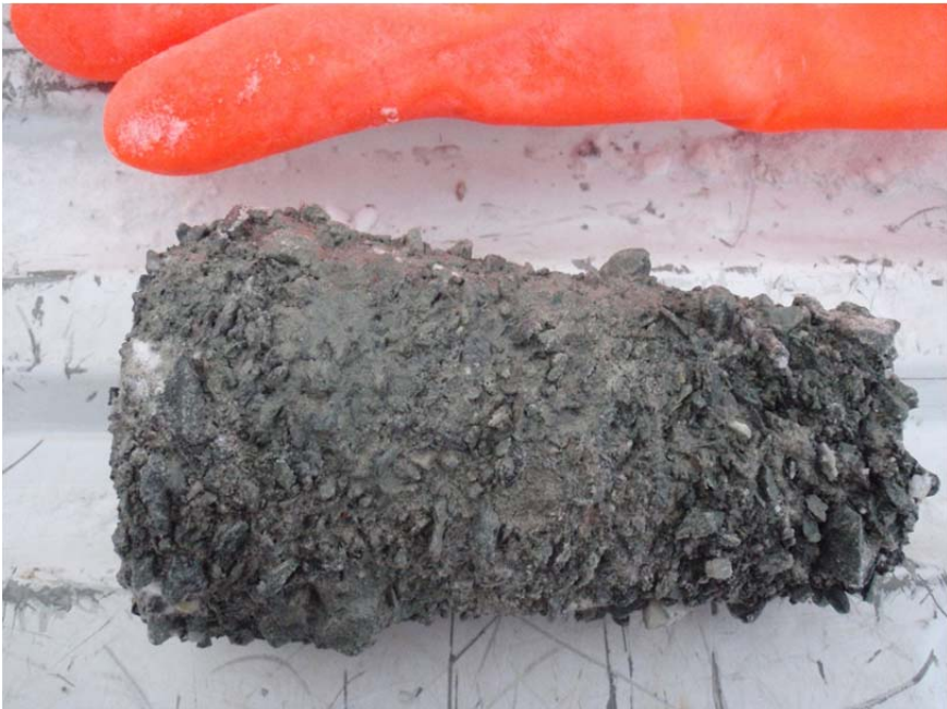
Photo 4: Drill core HB12-ND-CORE-DC-20-QA-20120204. Poor quality due to spinning gravel in barrel. Taken from 1+60 CL to upstream.
